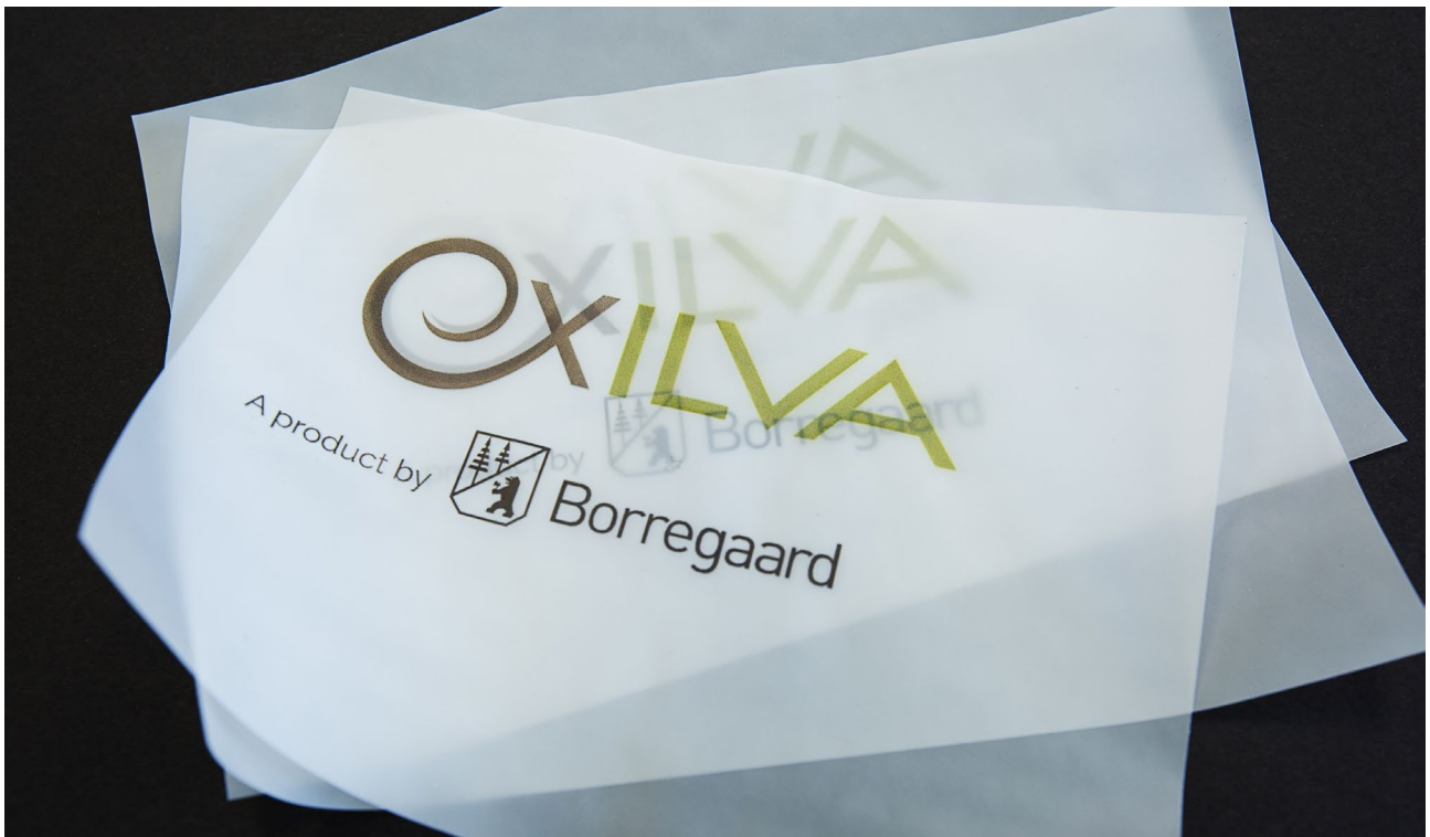
FIGURE 1: Exilva films made by casting containing 30% of sorbitol. The films are 35 \mu\text{m} thick and the printing has been made with ink-jet printing.
