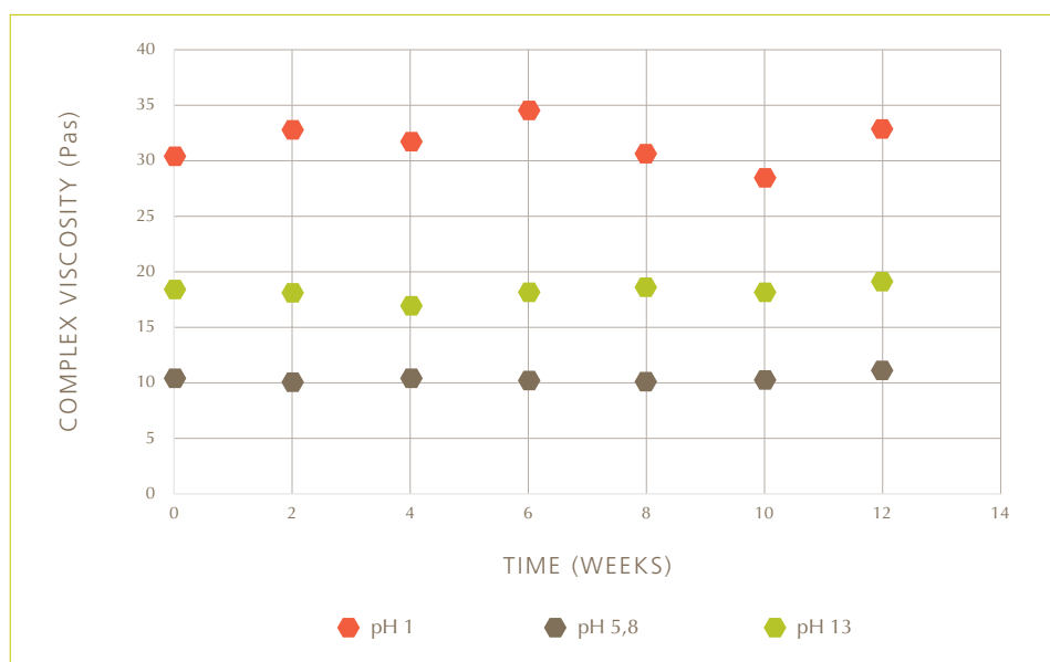
FIGURE 1: Complex viscosity of 1% Exilva suspension in water at different pH.
