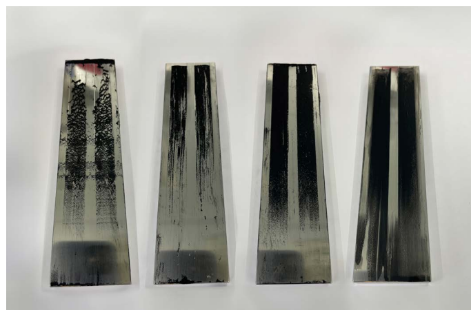
Figure 2: Hegman gauge demonstration of Super P C45 carbon dispersed with 0 wt% (left), 0.1 wt%, 1 wt%, and 5 wt% (right) Vanisperse LI at 5% solids in water.
