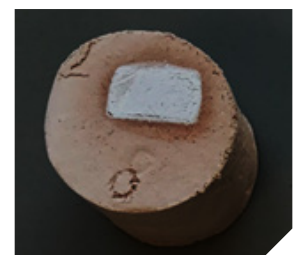
Example of fired product with no anti-scumming product available
