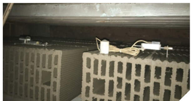
Monitoring tools used to track drying process
