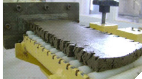
Low plasticity, cracked clay
