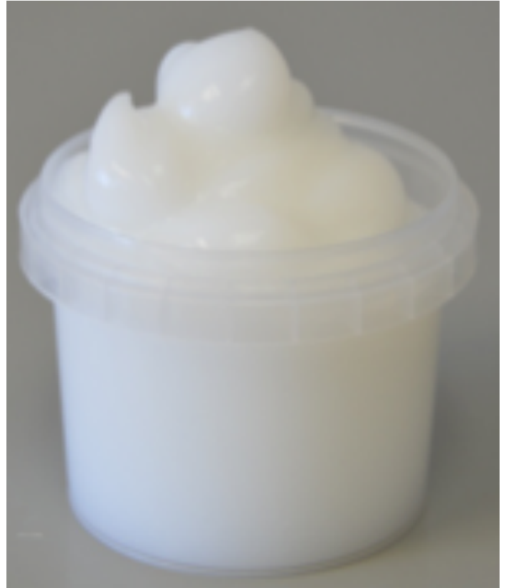
FIGURE 9 MFC can hold a lot of water compared to its mass. This picture shows 2% MFC suspension in water, which is creamy or gel-like even if it contains 98% water.
