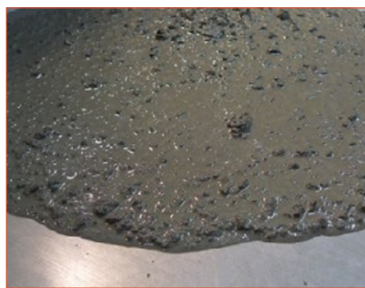
FIGURE 2. Concrete mix with 0.75 % lbwc of Exilva at initial spread.
