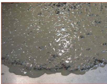
FIGURE 1. Reference concrete mix at initial spread.
