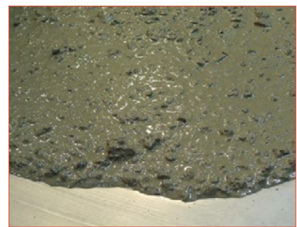
FIGURE 3. Concrete mix with 1.50 % lbwc of Exilva at initial spread.
