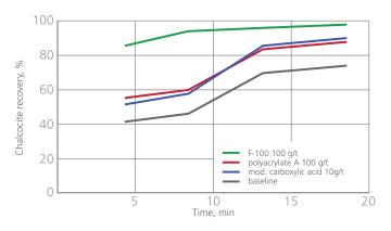
After the copper flotation steps, the activators,  $\rm Na_2S$  or  $\rm CuSO_4$ , were added together with PAX as collector. Pionera F-100 also improved the pyrite recovery and the associate gold in the flotation process. It is believed this is the result of de-sliming of the ore particles by the biopolymer.
