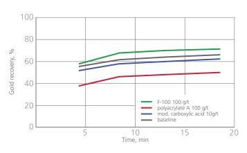
Figure 3: Flotation recovery in laboratory tests with different dispersants at their optimal dosage: pyrite
