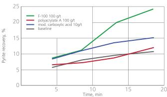
These positive results led to the planning of a plant trial with the Pionera F-100 to determine its effect on gold/copper recovery and clay. The product was tested at random over the course of 3 months.
