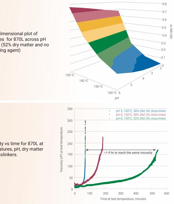
Figure 1. Three-dimensional plot of predicted gel rates for 870L across pH and temperature (52% dry matter and no added cross-linking agent)
